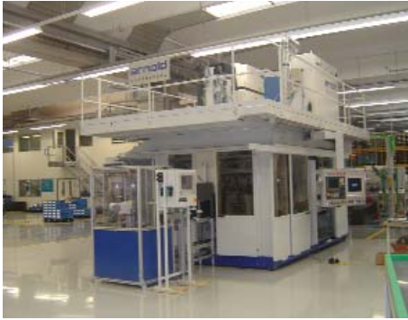
System for a laser welding process with filler material at ZF Gotha (System integrator Arnold, process development by IWS)
