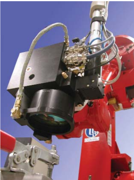
Fig. 1: Beam deflection optics lasertronic® SAO1.06 for the remote welding with high power YAG lasers
