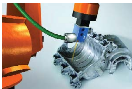
Nd:YAG laser based adhesive bonding surface prepossessing of an intake manifold made from magnesium in a high pressure die casting process
