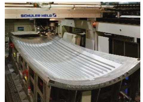
Fig. 2: Double-sided simultaneous welding of stringer skin field joints
